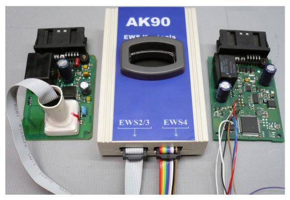
For EWS2,3 you have to clean the pins on the MCU for reading data . For EWS4 you only solder a 6 wires on circuit by following the number on the cable.
