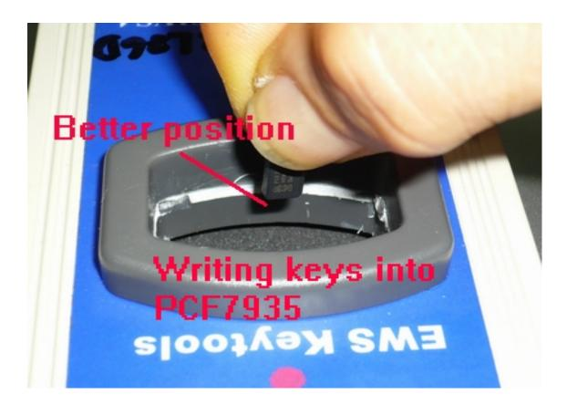
Waiting for 1 minute , do not move during programming Or the key will be failed in programming
