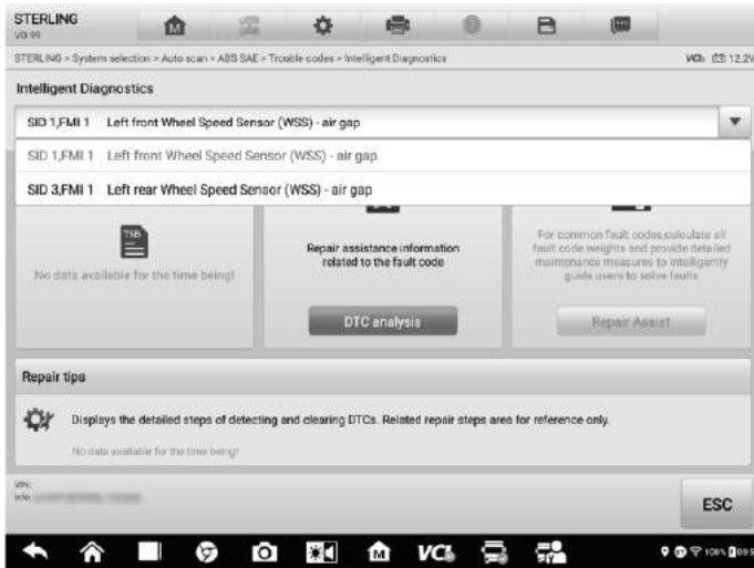
Figure 5-16 Sample Vehicle System and Detected DTC(s) Screen
