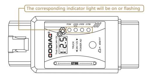
If you do not connect the car and only connect the diagnostic equipment for software communication signal test, you can judge whether the communication of the diagnostic equipment is normal.
