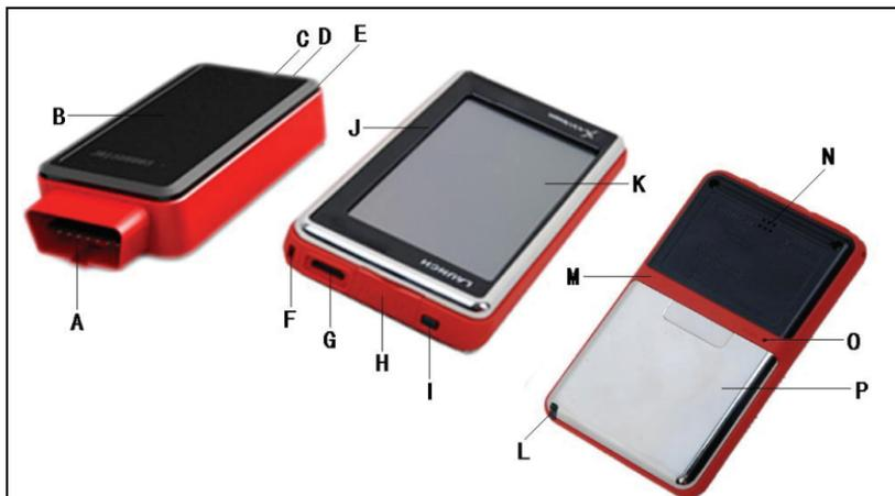
Figure 2-2 X-431Diagun main unit ports and indicators
