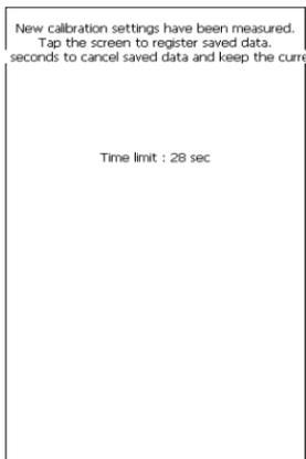
The screen will display interface as shown on the left after the touch screen was calibrated. You can click to enter the system desktop, or wait for 30 seconds to enter automatically.
