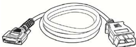
Figure 2-4 Main Cable – 1.7 m in length
