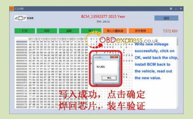
Part 7: Weld the chip 24C32 back to the BCM, install the BCM back to the car, start the car, it display 7372KM, the mileage correction succeed.
