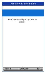
2. Input a valid VIN code and use the function key **Finish** to confirm. The scan tool starts to identify the vehicle.
