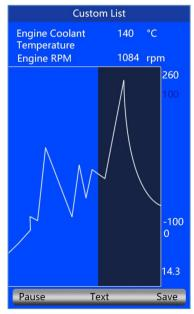
2. Press the function key **Two Graphics** to display two PID graphs in one screen.
