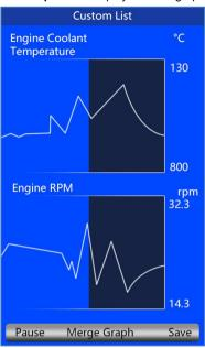
3. Press the function key **Merge Graph** to display two PID plots in one coordinate for easy and intuitive diagnosis.
