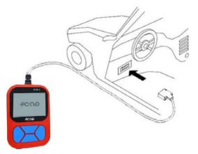
2 Take F501 for example (the operations for F502 diesel code reader is similar). After being connected to diagnostic socket, FCAR reader will start automatically and display the logo of FCAR. A few seconds later, you will enter diagnosis interface and choose the function you want. If you want to do diagnosis, please choose "Diagnostics" and enter it by clicking the key "Enter".
