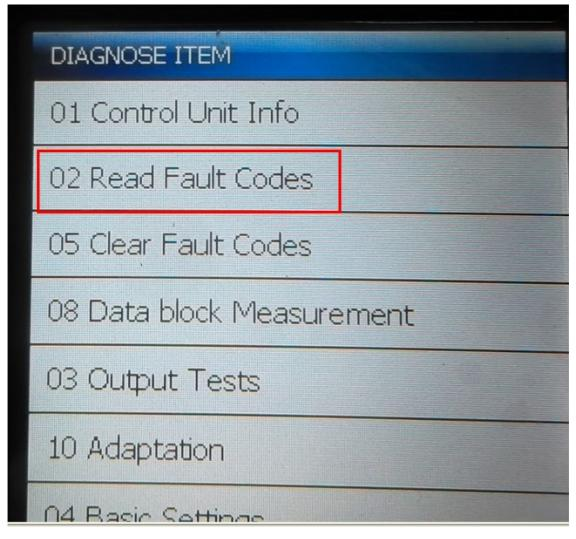
12故障代码读取成功 Successfully read out fault codes (DTCs)
