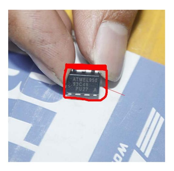
10, insert the chip in the right position and connect the OBP, (Note: notice 93C46 direction)
